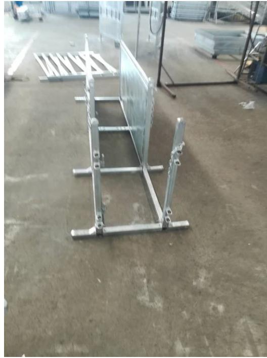
Above left and right, simple bolted walls together with the bottom brackets. Now you can tighten up bolts and make sure all are squared and correct angles. Below see next put the side gates on and lock the hinge pins with "Pin-socket". See the last picture do the same for end gate.
